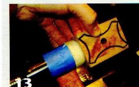
13 Test the fit with the cup itself.
