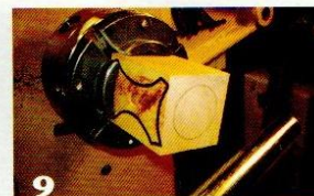
9 Mount the block into a 4-jaw chuck. On the end, scribe a circle the same diameter as the small cup.
