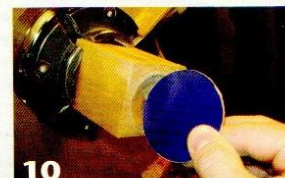
10 Use the template to test the diameter and depth of the concave area. The bottom of the ball (circle) should not touch the bottom of the concave area.
