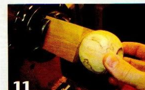
11 Use the ball to test that it does not bottom out in the hole. Flip the block over in the chuck and hollow out the other end to create the large cup.
