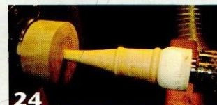
24 Finish-turn the base of the stick.
