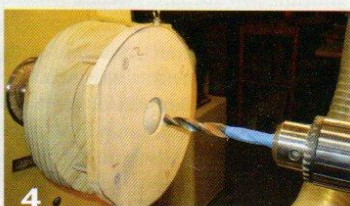
4 With the tailstock loose, push the tip of the drill bit into a small hole that you turned in the ball. Let the tailstock align with the hole, and lock down the tailstock.
