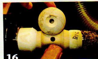
16 Use the ball itself to check for a good fit.
