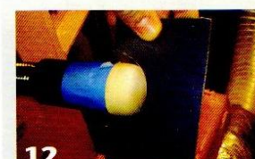
12 Turn a bung for use with the live center of your tailstock. Use the template to make sure the cup will fit onto the bung.
