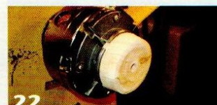
22 Use a scrap piece of wood, held in the 4-jaw chuck. Cut a flat on the face of the wood, then drill a \frac{3}{8} " (10 mm) hole into the wood.
