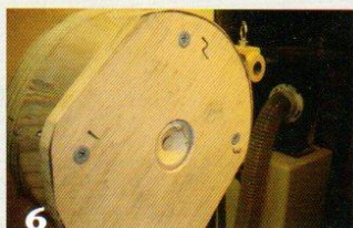
6 Turn a countersink around the hole.
