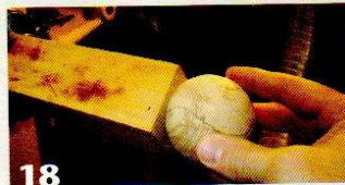
18 Hollow out the bottom cup and test-fit the ball.
