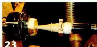
23 Mount the stick back onto the lathe. Use the bung for support.
