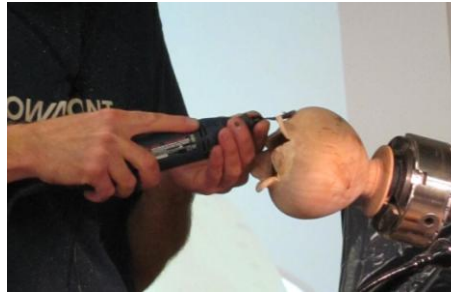
Detail shaping with Dremmel tool and small cutter
