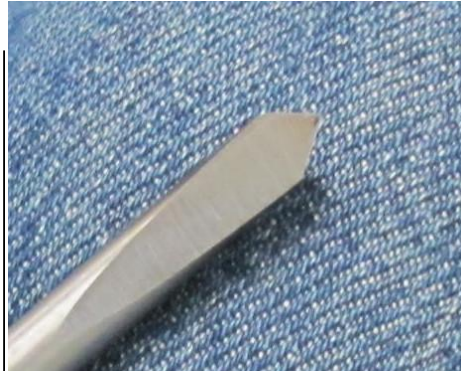
Diamond tip tool for cutting sharp "v"
