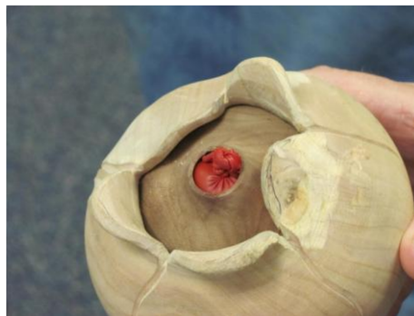
Insert held in place by a balloon to dry / eventually be glued into place
