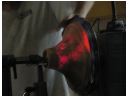
Light is run thru the head stock and inside the vessel
