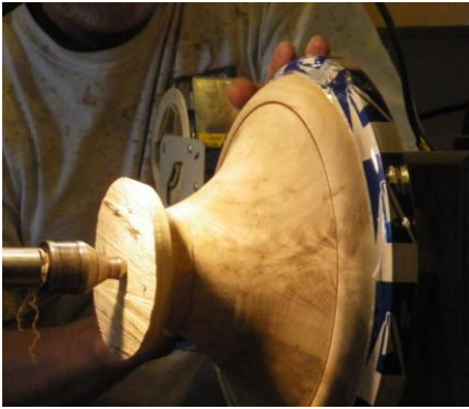
Attached to mdf with plastic tape
