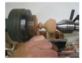
Use a "Texturing Tool" at 500 RPM to decorate the cap, (\$30-\$40 at Craft Supplies; I like 12 TPI. http://www.woodturnerscatalog.com/p/49/4528/Apprentice-Wagner-Texturing-Tool?term=texturing%20tools). Complete the stem; if necessary, reverse chuck the cap onto a jamb chuck to finish the stem. Part off. Apply finish.
