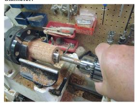
Using a 1 1/8" Forstner bit with a Jacobs chuck in the tailstock, bore out a recess about 3/8" deep, making sure to hold on to the chuck while boring or else it will tend to wander as it contacts the stock. You may want to use a small scraper to get rid of the
