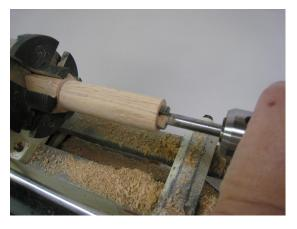
Now place a 3/4" Forstner bit into a Jacobs chuck, and bore into the piece remaining in the chuck, about 3" deep. Sand the outside smooth, perhaps to 220 or 300 grit. Mark the depth of the bore on the outside of the piece, about 3/4" to the left of the end of the bore, and then part it off. Remove the waste from the chuck.
