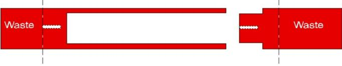
Once the majority of the piece is round, flip the ends and round the remainder, until the entire work piece is a cylinder. Standard #2 chuck jaws may be too big to hold the piece, so smaller jaws may be required. Alternately, a jamb chuck could be made to hold the work. Bring up the tailstock to support the free end.
