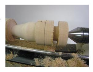
Round the area between the widest part of the scoop and the top of the cone, then between the widest part of the scoop and the tenon, and finally from the tenon to the end of the scoop. At this point, don't remove too much material from the scoop around the tenon, as we will refine that shape later on.
