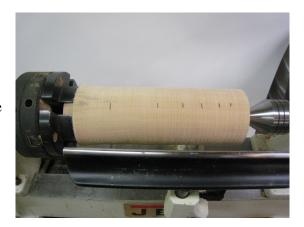
Using a Bedan or Parting Tool, reduce the size of the top of the cone to 2", and then cut a taper to form the bottom part of the cone. A sharp angle between the top part of the cone and the tapered part may be difficult to achieve, so don't worry if a small fillet remains.
