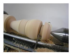
Using the hollowing technique of your choice, hollow out the main part of the scoop and cone; I use a Forstner bit in a Jacobs Chuck for the heavy hollowing. Size the entry such that it matches the tenon with a "Goldilocks fit", not too loose and not too tight, but just right (a small side ground square scraper would work well here, but a small parting tool on its side will also do the job).
