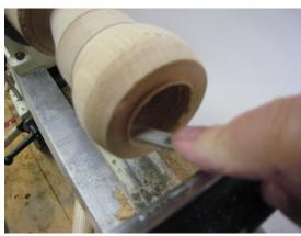
Place the cap into the body of the cone and refine the junction between the two parts; if the fit is a bit loose, wrap a piece of masking tape around the tenon while evening out this joint.
