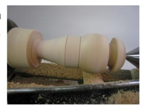
Making the box: Part off the top of the scoop, just about, but not quite, at the left side of the tenon (by leaving just a bit of the tenon on the main part of the scoop, we will have a rough idea of the amount of material to hollow to allow a good fit with the cap).
