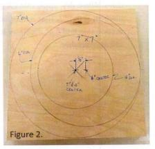
3. Mount it between centers using the small hole and round the outer 7" diameter. Mount it in jumbo jaws or a Longworth chuck with a thin backer board so you do not cut into the chuck (Figure 3) and carefully cut out the 4" circle with a parting tool, being careful to keep waste inside the 4" diameter. Cleanup to the edge of the 4" line with a scraper. Make sure that the cut is perpendicular to the face
