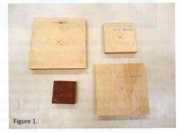
2. Draw a 7" diameter circle centered on the 7" plywood square. Draw a 4" concentric circle using the same center as the 7" circle. Drill a small hole through the center to mark the center on both sides. Use a drill press or make sure the hole is perfectly perpendicular. Mark a new center ½" off the center of the 7" diameter circle and draw a 6" circle using this offset center (Figure 2). Cut out the 7" circle using a bandsaw or jigsaw.
