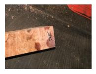
Turn side #2 up. Clamp it to the miter gauge and stop. Make another cut.
