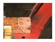
Glue an insert in place and clamp, as before.
