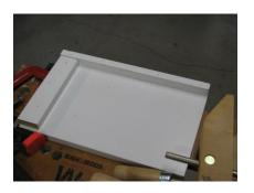
Spread wood glue on the insert and in the slot.
