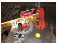
Set the table saw blade to cut <u>almost</u> through the base block. Leave about 1/8" of wood.
