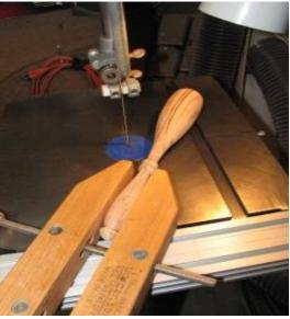
Use the band saw, with a fine tooth blade, to saw away the scrap and form the blade.
