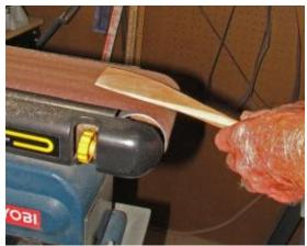
The curved end of the belt works nicely on the upper surface of the blade and the flat part of the belt works well on the bottom of the blade.
