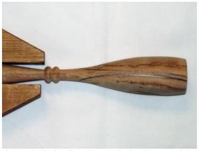
Clamp it by the handle with a wooden hand screw and draw the blade shape on the "club" with a pencil. The blade should be a little less than ¼" thick, with a slight curve, and flow smoothly into the shaft.
