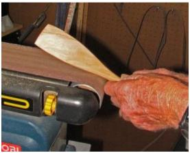
The belt sander and a sanding block finish smoothing the blade and flowing it into the shaft.
