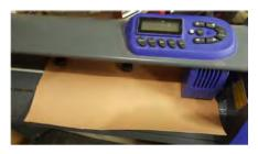
Sandblast resist or mask allows you to cover an area and protect it from the sandblast media. We'll discuss various vendors and mask products. Using the sandblast resist or mask can be done as simply as using an exacto knife and cutting out various shapes. I use a vinyl cutter (aka plotter) for this along with a software package – "Sure Cuts Alot". The vinyl cutter came from USCutter at uscutter.com. It is
