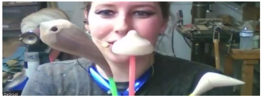
Straws make handy holding fixtures for applying finish. Deft lacquer satin is sprayed as a finish and the straw stuck in a bucket of rice to hold item until dry.
