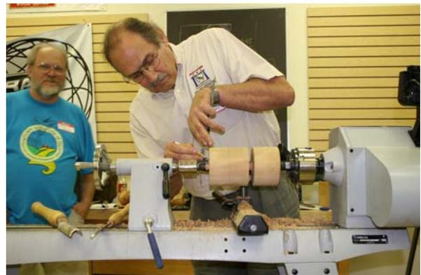
Next use a gouge to connect the lines you just drew creating an octagon shape. You should try to make your cuts flat from one line to the other with no dip or ridge. Use a straight edge to check it.
