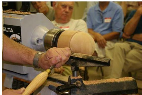
Now turn one half of the sphere down using the score mark as your guide. When you just make contact with the score mark you're done with that side. Flip the sphere around and do the same for the other half.
