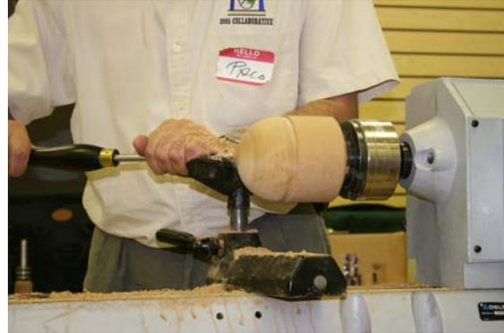
Now score the sphere just enough to touch all the way around on the line you just drew. This scoring mark will be a guide for the finished size. After scoring remove the sphere and re-install it orientated with the original center line vertical. (same as when you turned the cylinder)
