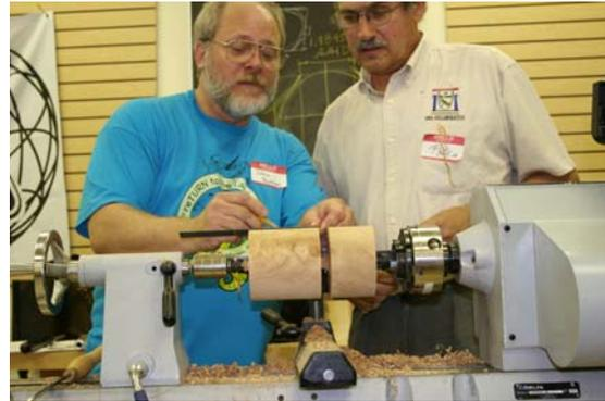
To begin turning a sphere you must first turn a cylinder slightly larger than the diameter of your finished sphere. It is best to use dry wood to prevent cracking. Now get out a calculator and write these numbers down. Take the radius (half of the diameter) of your cylinder and multiple it by .586.
