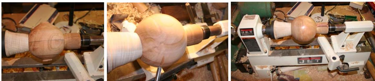
cylinder was 4.60 inches and the goal was a sphere 4.5 inches in diameter. One of the spheres was turned oblong to illustrate the effectiveness of the cup chuck method. The first sphere ended up at 4.54 inches and the second, oblong one, ended up at 4.29 inches. Good Luck!!!
