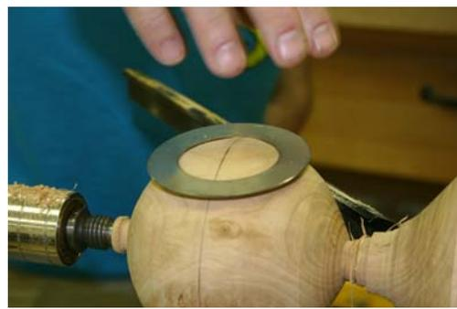
Once you have it close enough, part it off and make a jam chuck to hold the sphere. It is important that less than half of the sphere is inside the chuck.
