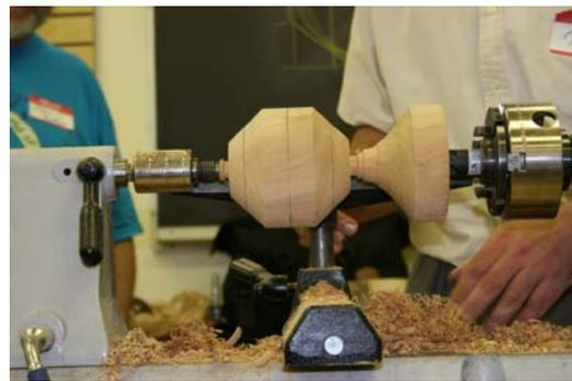
As your sphere begins to take shape you can use a large washer, a router insert or other flat donut shaped item to check for high spots. If your shape is perfectly round the washer will touch all the way around the inside edge. Mark high spots and turn them down. It is not necessary to have a perfect sphere at this point. Small ridges will be cleaned up later. Get it close and move on to the next step.
