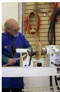
Start the top side by turning it true. Then begin to shape it from outside in, measuring as you go. Keep the tailstock in as long as you can, for additional support. When you can't go any further, pull the tailstock away for full access to the top of your
