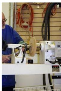
Now shape the outside bottom of the platter defining the rim. Once your happy with the shape stop the lathe and flip the platter so you can work on the top side. Bill has made a plastic "shoe" for his live center point. This allows him to use the tailstock to hold the platter flat against the chuck after reversing without damaging. He tightens the tailstock to hold the platter flat against the jaws. As he tightens the jaws, it centers itself on the tenon.
