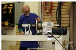
Bill chose to turn a piece of bird's-eye hard maple, a difficult wood to turn due to its varying grain direction. When determining what side of the blank should be the bottom or the top find the side with the most figure. Once you identify the most appealing side, make that the bottom. When turning the top side you will turn through the less desirable wood and the better figure will show up in the bottom of your platter.
