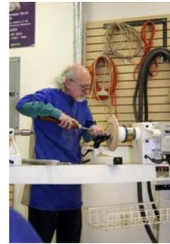
Reverse chuck the platter using your preferred method (vacuum, cole jaws or friction). Bill uses a vacuum chuck, which allows full access to the bottom. Finish shaping the bottom and remove the tenon. Sand through all the grits and apply the finish of your choice.
