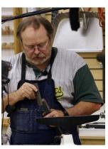
grain smoothly. Alan made one from scratch in very little time and explained the process thoroughly. He even covered what the steel was going through and defined the terms annealed, hardened and tempered. 4 hook tools can be made from one \$3 piece of drill rod. Many members showed interest in getting together for a
