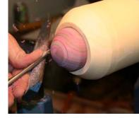
Now assemble your box with the grain aligned then rotate the lid 90 degrees from the base. This way when our box is complete we will rotate the grain back into alignment when in the drunken position.
