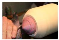
lathe running. This is your indicator for having the box properly installed into the chuck. Once that is done create a straight cut that will eventually go from the dots you drew to the dead center that shows when the lathe is running. Make multiple passes and try to make the cut as straight and accurate as possible. The goal is to create this flat area without changing the
