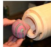
major diameter of 60mm. Once done, remove the box and create a jam chuck to reverse the box and do the same on the other side.
