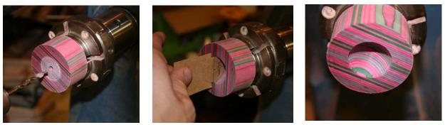
interior. A <sup>1</sup>/<sub>2</sub>" round nose scraper works best. Stop often and check the circumference and shape with your positive 30mm template. Take your time as you reach the bottom of the pre-drilled hole. Continue to
