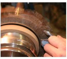
few passes to check that the wing is square to the lathe, a small ruler works well for this. Slow movements are important since the wing is irregular and you will be cutting through air at some point of the wing. Once the top of the wing is square and smooth you can begin on the other side of the wing. Do not try to sand the wing while the lathe is moving. Since the edge is irregular you may have a catch which will break the wing or possibly hurt you. I always hand sand the wings of these bowls.
