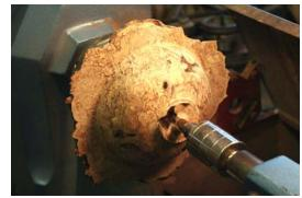
Install your bowl into the chuck and clean up the facing surface. If you need to extend the size of the wing to match the size on the other side, do this first. Do not try to re-cut the edges of your wing from earlier. The wood has probably moved too much and it is too thin to change. Once the face is smooth determine the inside edge of the bowl. If you want to place a detail to define the edge of the bowl itself, do it now. This could be a cove, a bead, a v-cut, or even just a raised lip.
