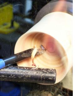
bent (above left). Then reheated to above critical temperature in the forge (above right). Lastly, it was quenched in oil to harden it. The last steps were to be done at home. That is, tempering for 30 minutes at 450 degrees so it would be tough but not brittle and grinding the final edge. At left is shown a test run using one of the hook tools on end grain, the perfect application for this tool because it cuts the grain smoothly as opposed to a scraping cut. It worked great.
