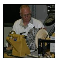
Bill believes the best way to mount the platter for turning after incising is onto a large flat jaws chuck. Neat Stuff!
