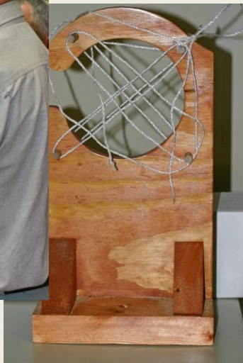
Unique design for a steady rest used for turning long, thin finials.
