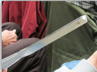
Although Dave called this his "double skew" it is actually a tool he made to clean up the corners of mortising cuts in the timber furniture he is making.
