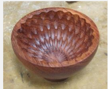
Box and bowl turned and then decorated with a Rose Engine by John Buehrer. Decorating the inside was a real challenge.
