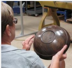
Michael Blankenship created this walnut bowl and finished it with 10 coats of polyurethane and a final coating of buffed wax.
