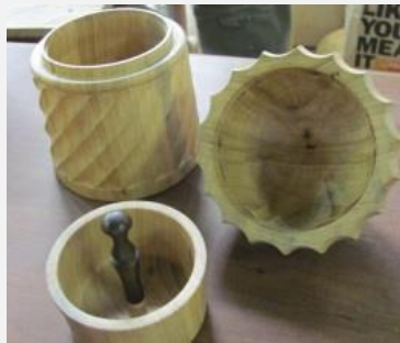
Box and bowl turned and then decorated with a Rose Engine by John Buehrer. Decorating the inside was a real challenge.
