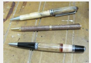
Pens turned by Jan Hoffman and the jig she designed to hold the pen blank while drilling. The top pen is silver maple with a CA finish, the middle pen is mahogany with a Briwax finish, and the bottom pen has a Shellawax friction polish finish.
