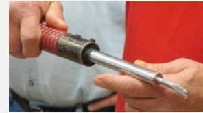
Hook tool made by Dan Schmoker. The tool is introduced to the turning slightly below center and then raised.
