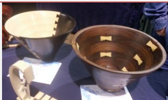
These bowls were NOT turned. They were made with a scroll saw set at an angle, cutting each ring from flat stock. You can see the blank below one of the bowls on the right.
