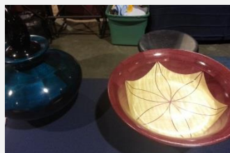
These bowls were NOT turned. They were made with a scroll saw set at an angle, cutting each ring from flat stock. You can see the blank below one of the bowls on the right.
