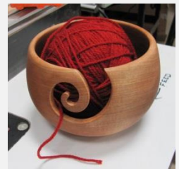
Walt Ahlgrim turned a yarn bowl for his wife and used a spiral cutting blade on a jig saw to cut the curve for the yarn. He is also shown in a hockey mask that he purchased to use for a face shield while turning.
