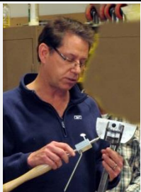
Steve White with a fixture he made to sharpen a spindle tool made by Cindy Drozda . The offset holes allow you to quickly grind a secondary bevel on the tool. Steve also showed the jig he made to cut thin slots in his Christmas ornaments which were then filled with a veneer before final turning. The other enhancements were added with his Rose Engine lathe.
