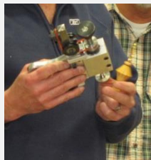
Steve White with a fixture he made to sharpen a spindle tool made by Cindy Drozda . The offset holes allow you to quickly grind a secondary bevel on the tool. Steve also showed the jig he made to cut thin slots in his Christmas ornaments which were then filled with a veneer before final turning. The other enhancements were added with his Rose Engine lathe.
