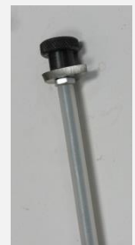
Lloyd Richardson made this fixture to hold small HSS cutters for sharpening.
