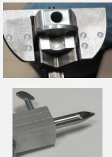
Steve White with a fixture he made to sharpen a spindle tool made by Cindy Drozda . The offset holes allow you to quickly grind a secondary bevel on the tool. Steve also showed the jig he made to cut thin slots in his Christmas ornaments which were then filled with a veneer before final turning. The other enhancements were added with his Rose Engine lathe.
