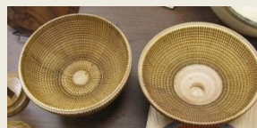
Dan Burleson beaded vessels. He brought one that was in-work to show the process for beading the interior. It is turned as two “bowls” then joined with a tenon that is “one bead wide”. The painted pattern from the outside is echoed on the inside before joining.
