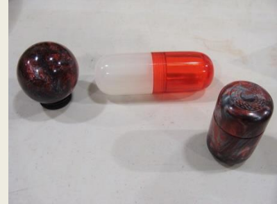
Jeff Hornung – Acrylic Resin Pill containers with manually cut 16 tpi threads
