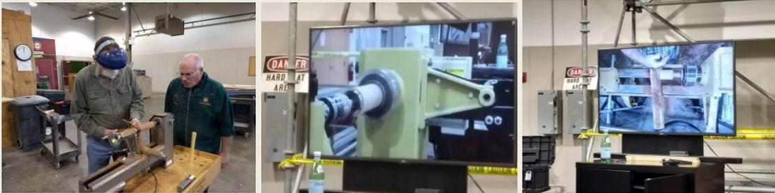
John then began to turn the handle. He rounded the outside of the scoop into the handle. He then used a beading tool to add a decorative element at the intersection of the scoop and the handle. John used Yorkshire grit finish with beeswax. Lastly, he used a belt sander to shape the scoop. Below are a couple of videos on turning a scoop.
