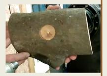
Note: Check the clearance of the piece – over the bed and over the banjo before starting. Level off the bottom, define tenon, and start shaping the bowl.
