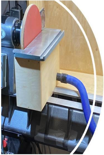
Richard Grossman – Lathe driven disc sander
